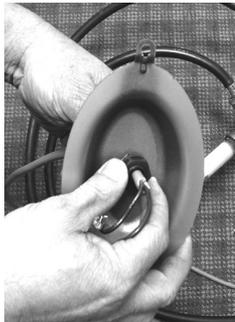
Screw the retaining ring onto the back side of the cover, hand tight. This will hold the cord in place on the cover.
