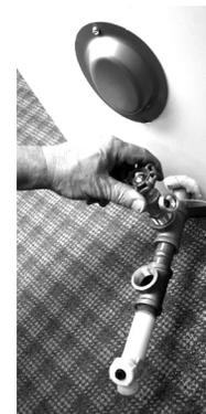
Next, apply thread seal tape to, and install a valve, (item 104), onto the "T" fitting closest to the tank, making sure it is tight.
